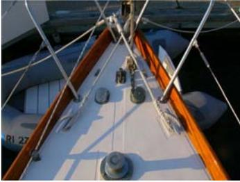
The T34 has a very fine bow and, as such, anchoring hardware has to be planned and installed carefully. Here are installations from around the fleet to consider when upgrading or revising your equipment.
