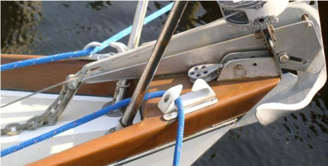
the bow roller - instead I had fabricated a SS strap bent in an S-shape to support the roller tail on the deck.
