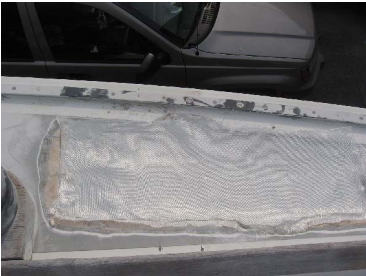
Port forward stanchion area - core removed and edges beveled - ready for recore.
