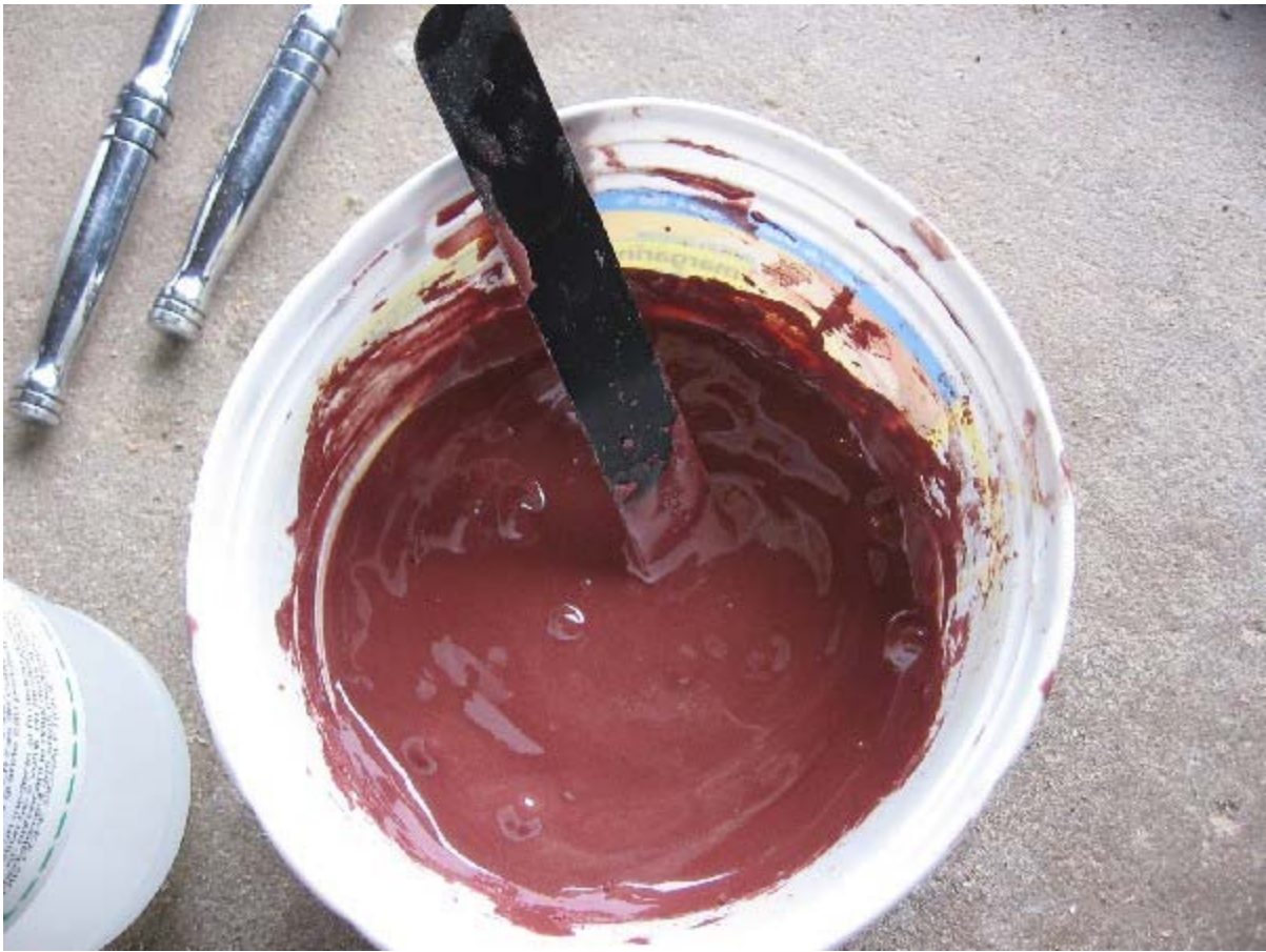
Epoxy mixed with Sandable Filler for skim coat
