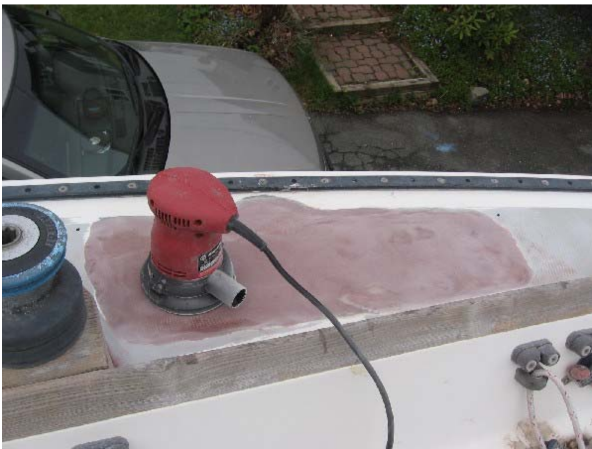
Sanding the high spots using 80 grit and Random Orbital Sander
