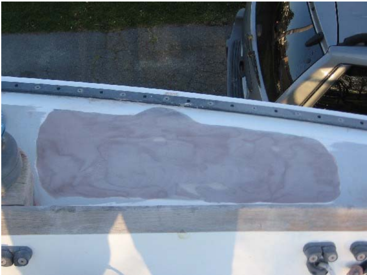
Port aft - ready for primer & paint
