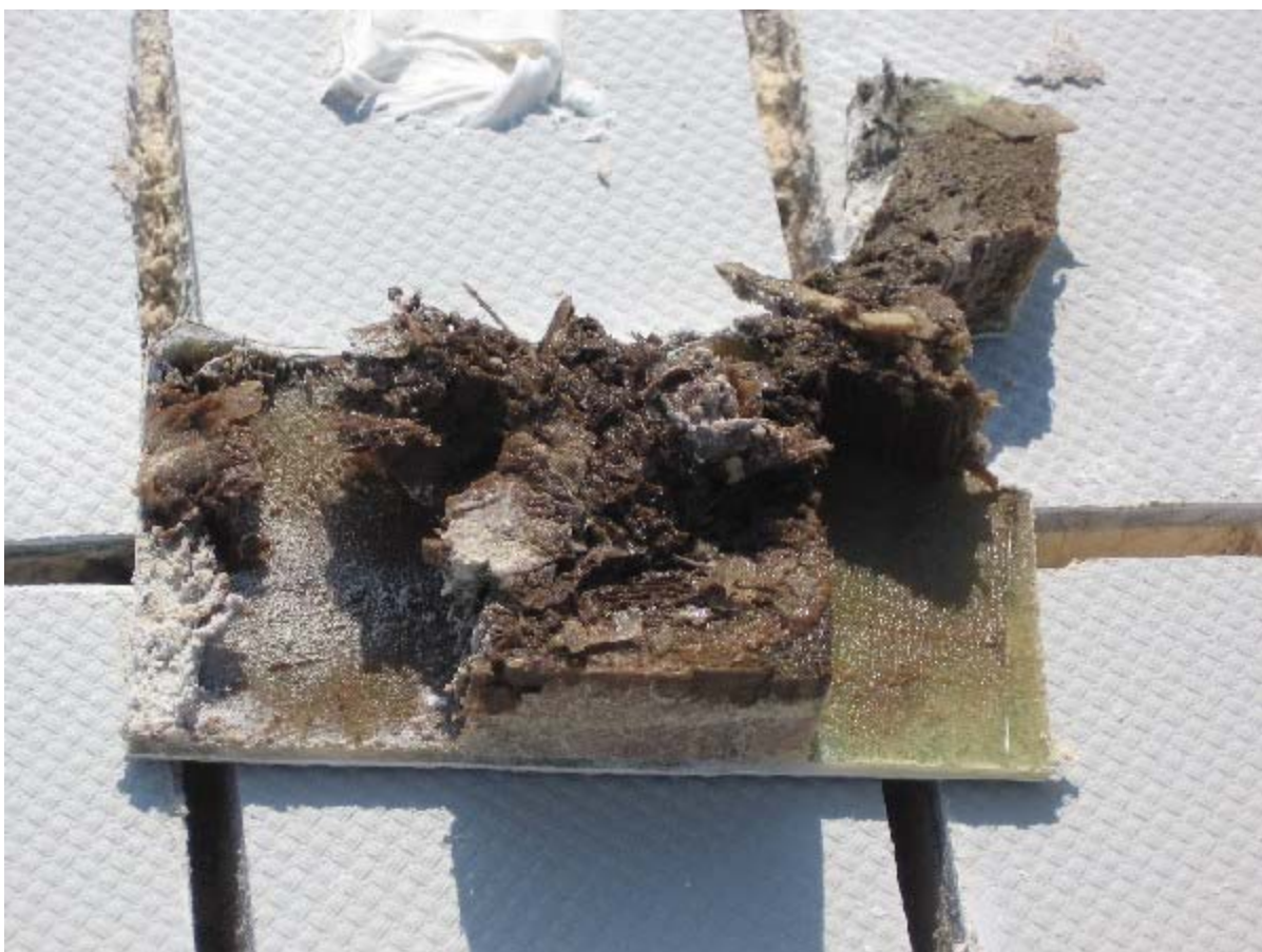
Removal of old core. Using wood chisel and hammer.
