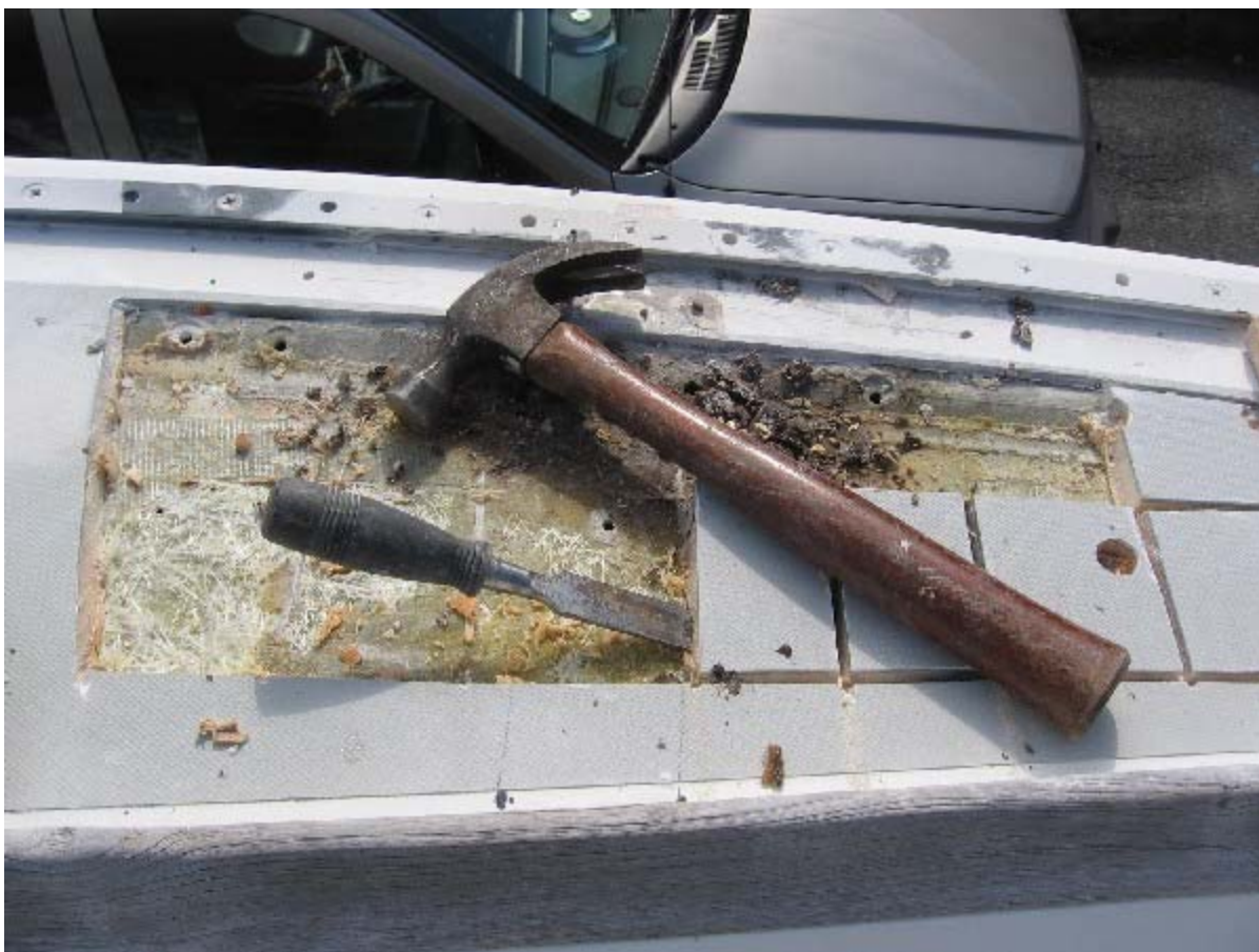
Removal of old core. Using wood chisel and hammer.
