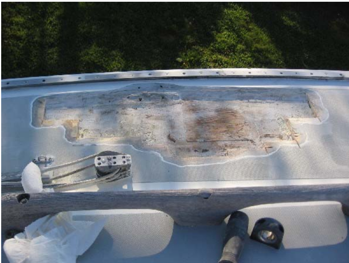
Port forward stanchion area - core removed and edges beveled - ready for recore.
