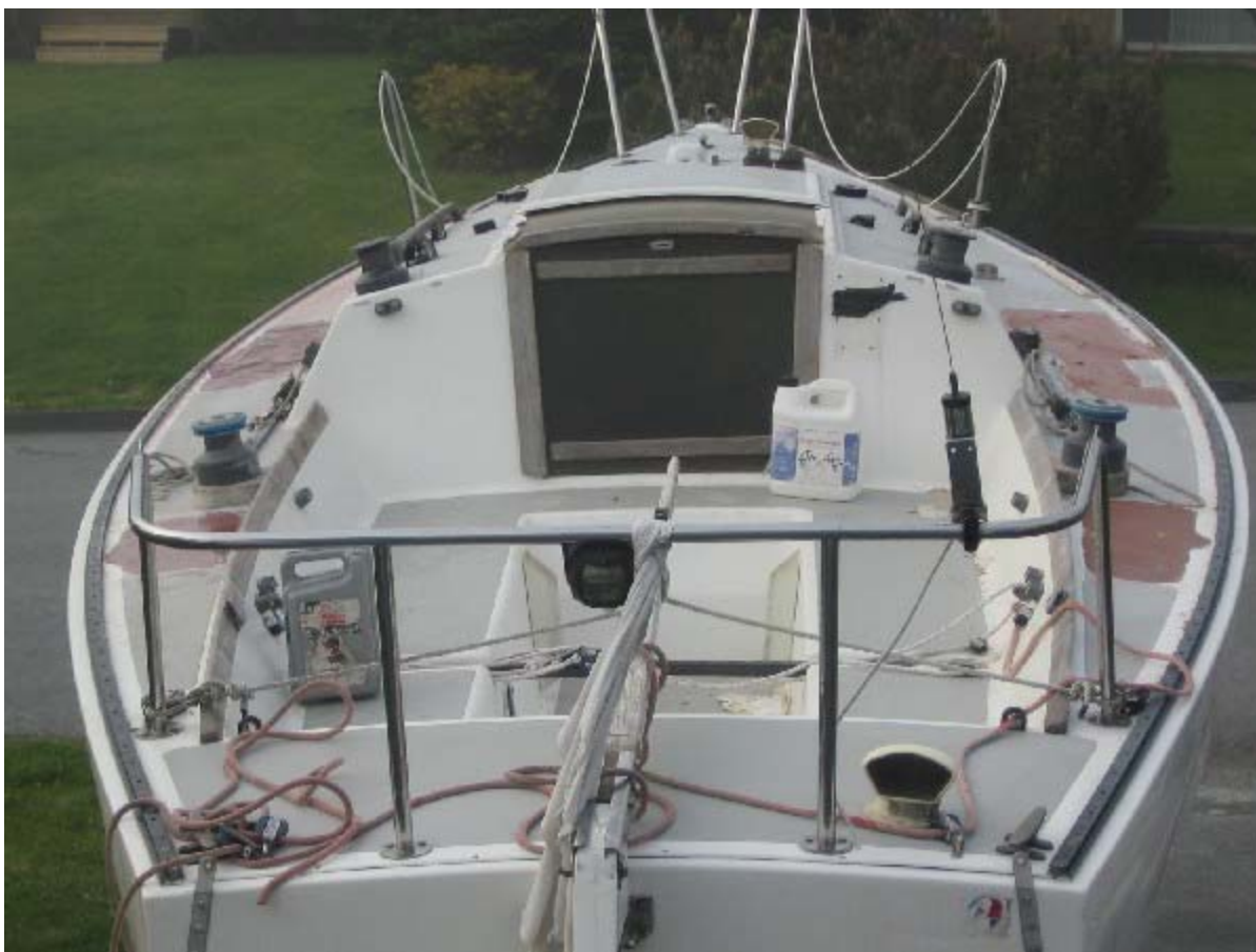
All four sections now recored and fairing coats applied
