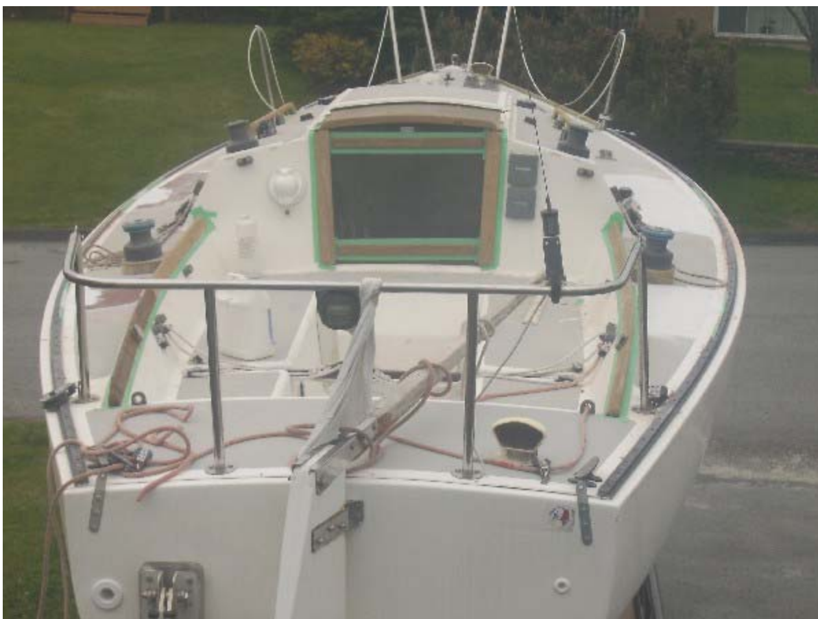
All four sections now recored and fairing coats applied
