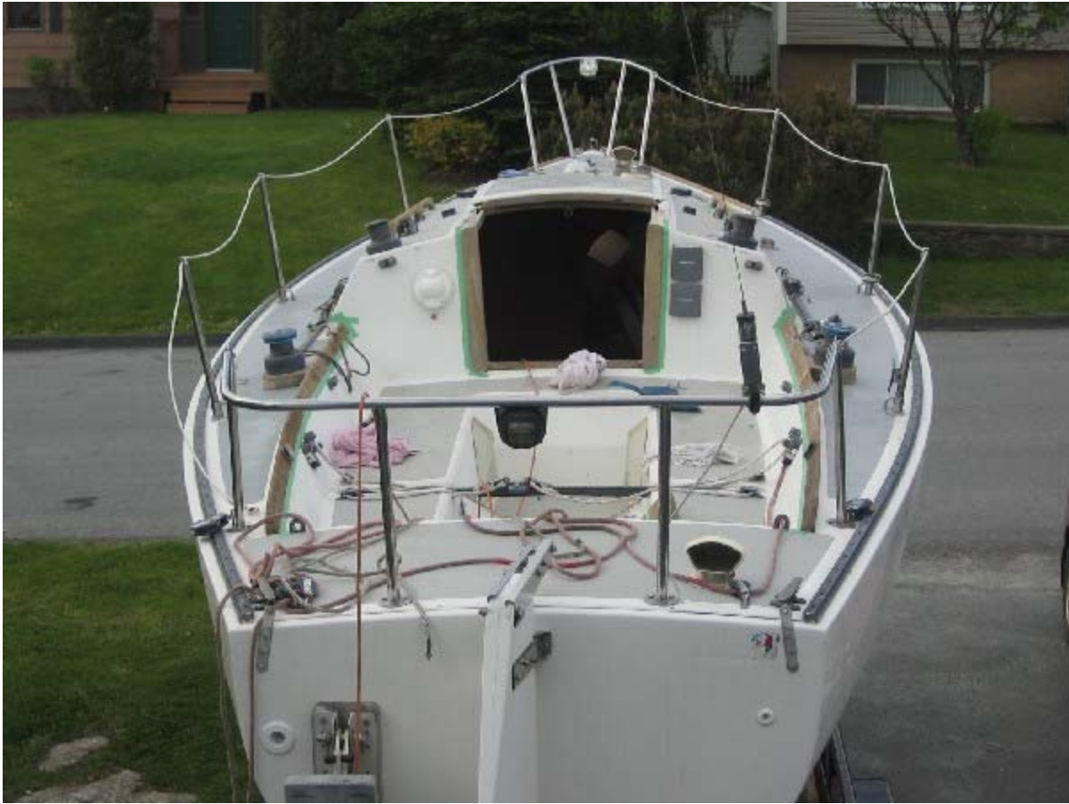
Job Complete with stanchions rebedded. Forgot what a pain that was!
