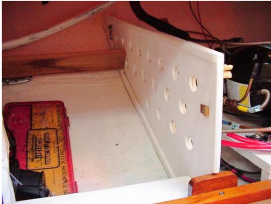
To finish the compressor installation, I built a plywood partition for the locker. This keeps anything stored in the forward half of the locker from tangling with the machinery in the after half. The partition can easily be removed to provide access for maintenance.
