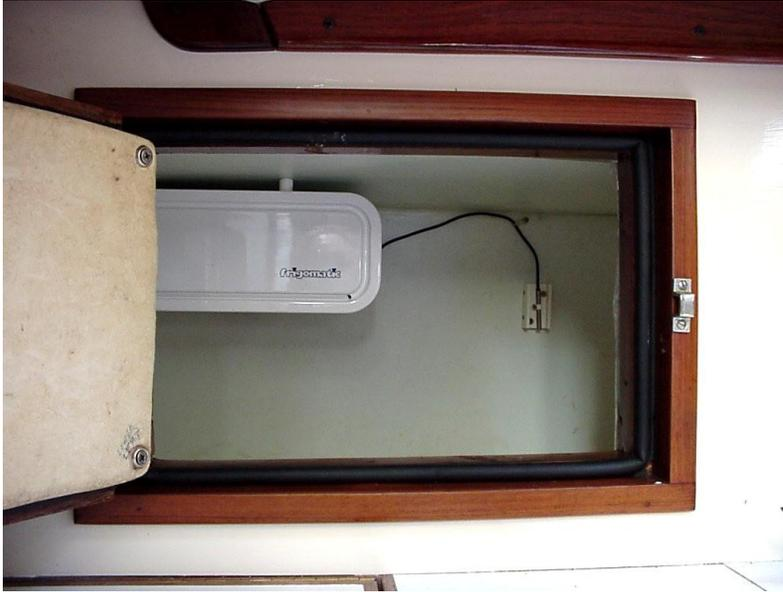
The muffin fan (mounted to the box's ceiling in the forward, outboard corner) is connected to the compressor power supply and turns on whenever the compressor is running. It gently tumbles the air inside the box, blowing it across the evaporator and improving the heat exchange efficiency.
