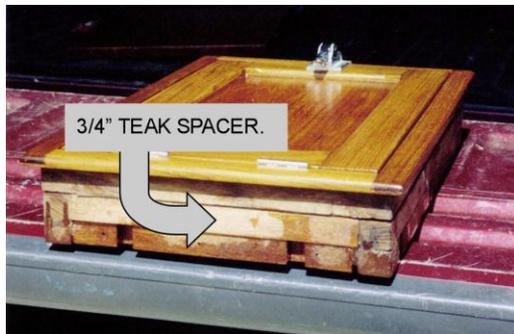
The increase in depth of the doorframe allowed me to add a piece of Tuff-R on the inside of the door, under the molded fiberglass insulation panel. I also replaced the door gaskets with a "P" type gasket on the frame that compresses into a twin hollow gasket on the door and makes a very airtight seal.
